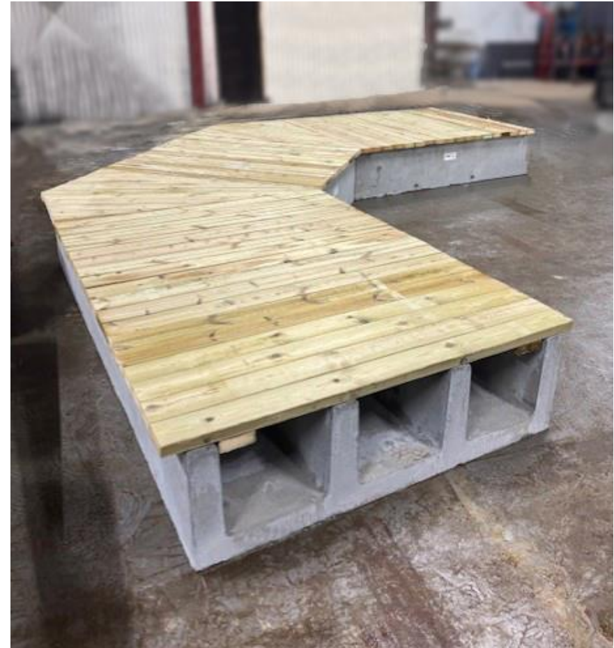
Troughs with wooden covers in the factory.
